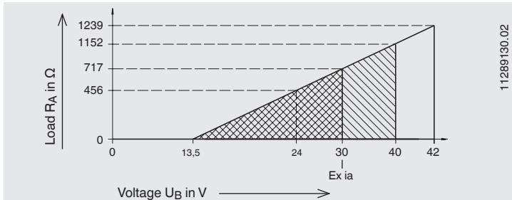
For the power supply, use an energy-limited electrical circuit (EN/UL/IEC 61010-1, section 8.3) using the following maximum values for the power supply:
